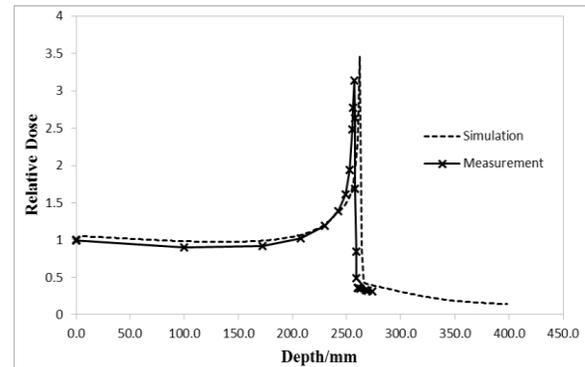
**Figure 2 (b):** Depth dose distribution (Bragg peak) of carbon ion beam for measurements and simulations with 400 MeV/u
