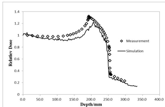
**Figure 4 (b):** Depth dose distribution (SOBP) of carbon ion beam for measurements and simulations with 400 MeV/u
