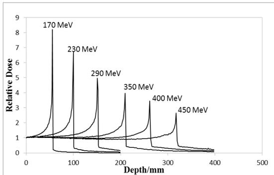
**Figure 3:** Depth dose distribution of carbon ion beams in water at various low energies by Geant4 simulation
