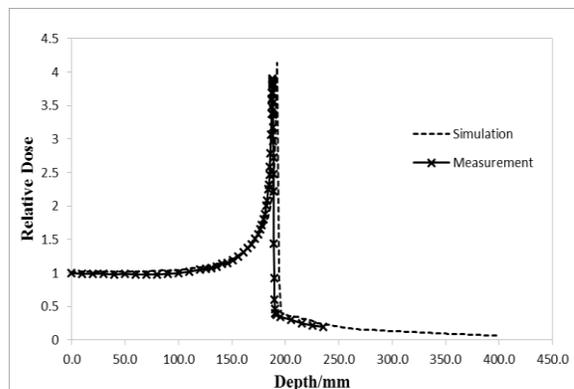
**Figure 2 (a):** Depth dose distribution (Bragg peak) of carbon ion beam for measurements and simulations with 350 MeV/u
