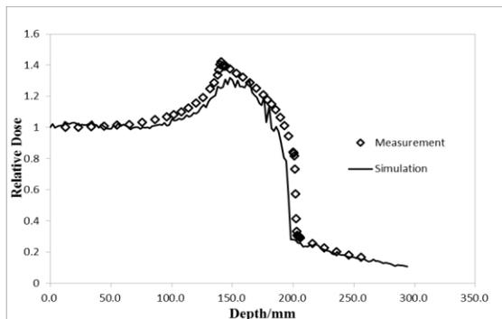
**Figure 4 (a):** Depth dose distribution (SOBP) of carbon ion beam for measurements and simulations with 350 MeV/u
